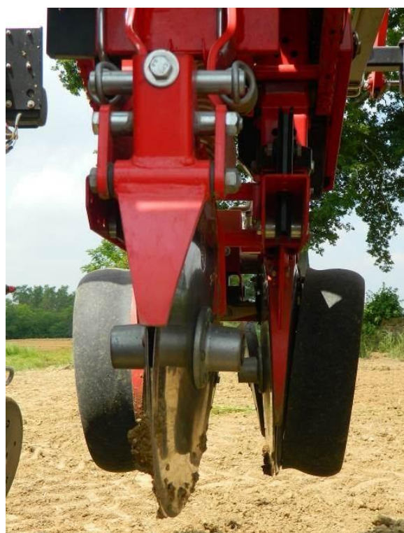
Fig. 7 – The planting elements of MS Twin will be supplied off-the-rack with double disc opener for fertilizer
