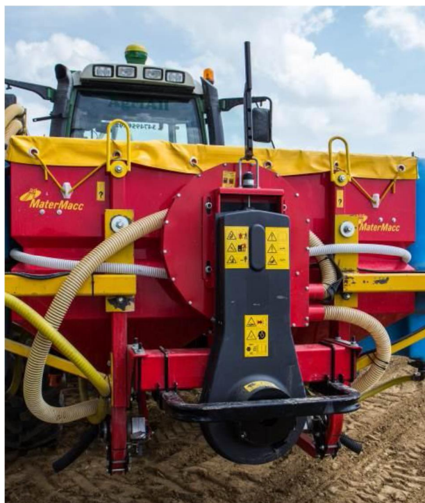
Fig. 4 – Among the available accessories for the Matermacc MS TWIN there is the Variovolumex fertilizer tank, with a capacity of up to 1300 l; the transfer of mineral fertilizer to the planter dosers is carried out by a pneumatic conveyor, whose fan is started
