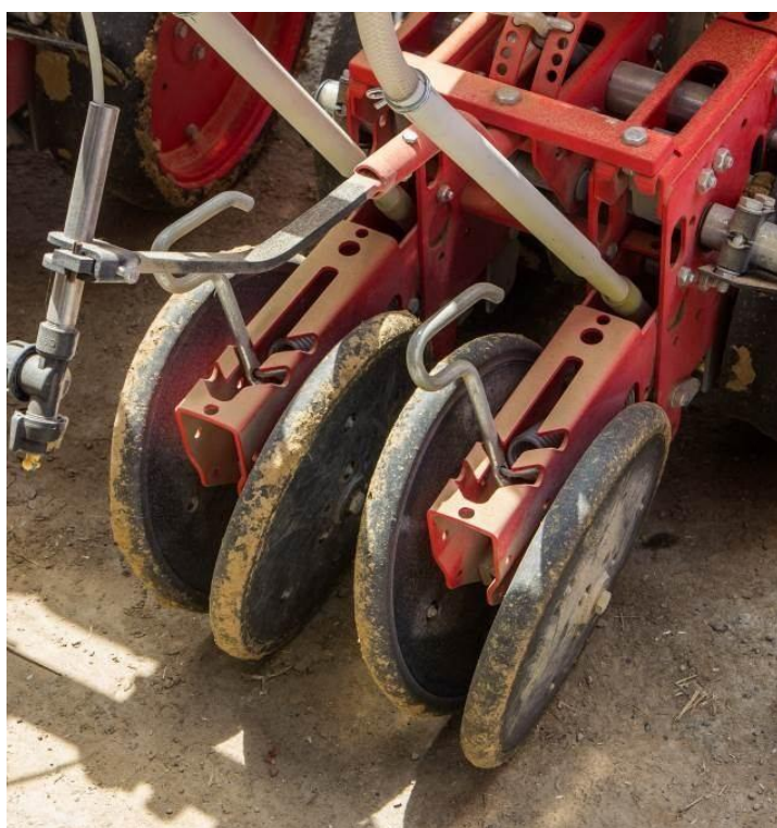
Fig. 6 – The rear wheels close the furrow, leaving a compacted soil
