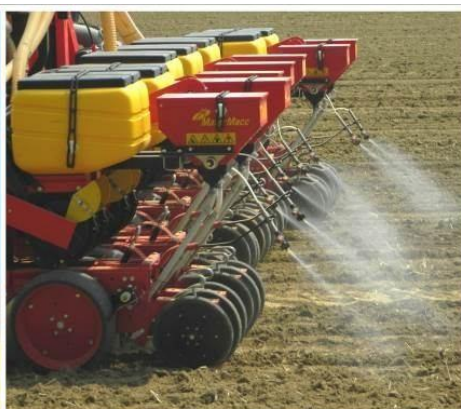
Fig. 10 – On each Twin element are assembled two independent seed hoppers with a capacity of 35 l each.
